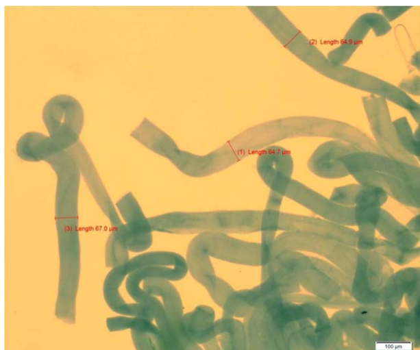
Figure 3. Swollen degummed dyed RB5 dyed fibroin in CWE after 2 h at 60 °C (scale bar 100 μm). [Color figure can be viewed in the online issue, which is available at wileyonlinelibrary.com .]
